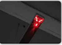
When a parking space becomes available, the occupancy status is updated in real time. This allows vehicles looking for parking spaces to quickly visualize the exact location where there is an available space. The time saved in looking for an available parking space can be used by customers to conduct their planned activities making parking a quick process.
